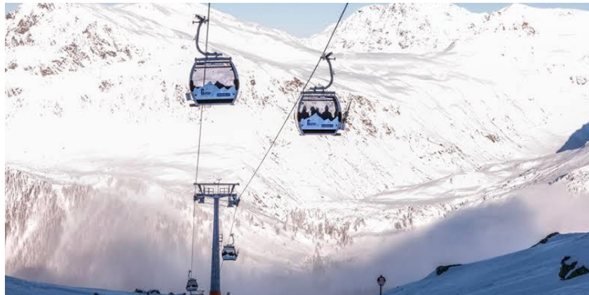
Continuously Moving, Mono Cable, Detachable grip type ropeway system
